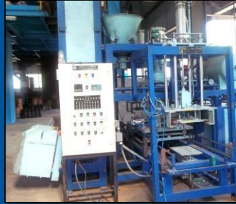
Horizontal Cold Box Core Shooter Double station – 10 kg & 20 Kg
