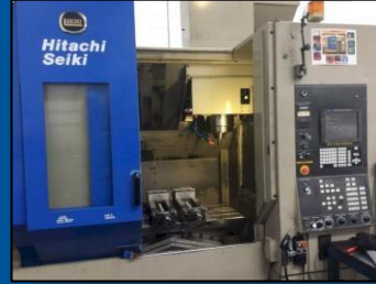
Horizontal Milling Center with auto probing
