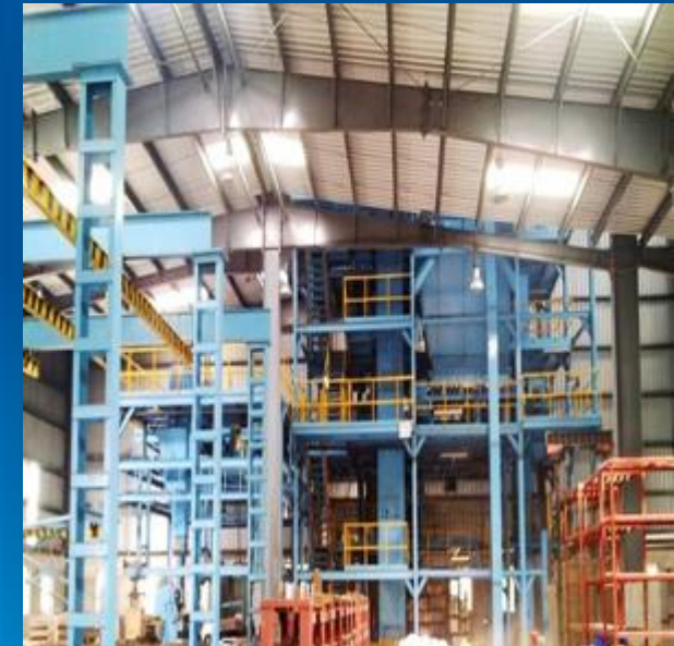
Fully Automatic Sand plant with 30 MT/hour Sand Handling system
