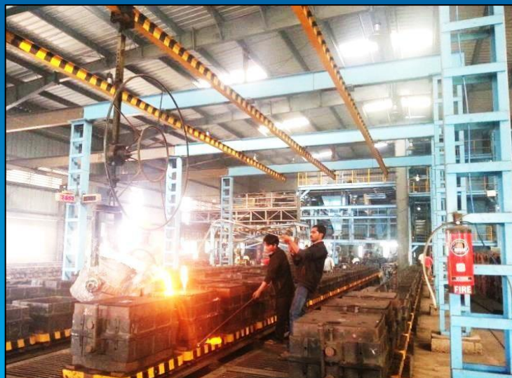
Molten Metal pouring through Monorail
