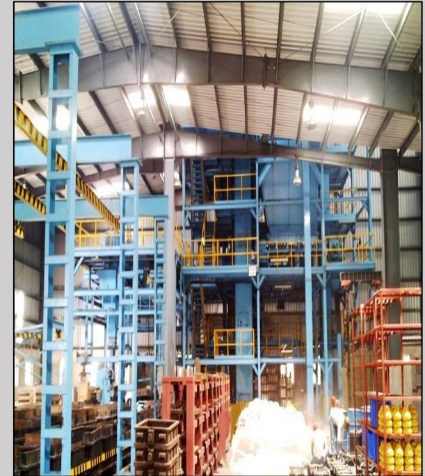
Fully Automatic Sand plant with 30 MT/hour Sand Handling system
