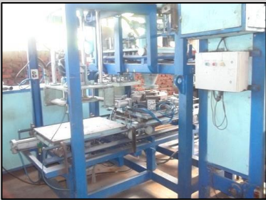
Vertical Cold Box Core Shooter - 30 kg
