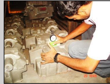
Core Scratch Hardness Inspection
