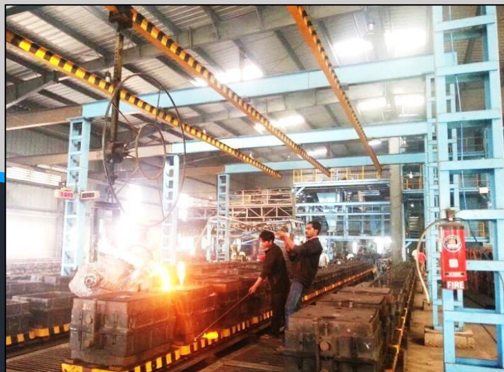
Molten Metal pouring through Monorail
